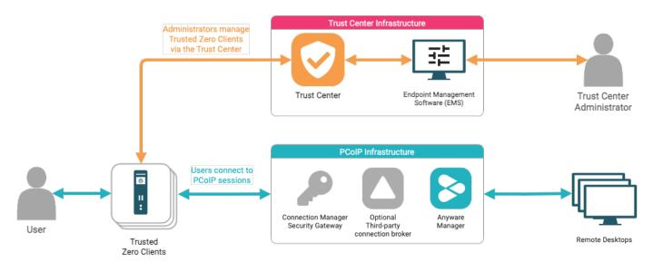
The Anyware Trust Center is an application composed of multiple services on a single VM. It connects to Trusted Zero Client endpoints and your Endpoint Manager.
